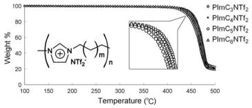
Thermal gravimetric analysis of the proposed polymerized ionic liquids.
